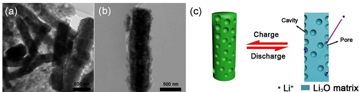
**Figure 10.** (a, b) TEM images of the  $\text{Fe}_2\text{O}_3$ -500 electrode after 50 cycles at a current density of  $500 \text{ mA g}^{-1}$ . (c) Schematic illustration of the charge/discharge process of  $\text{Fe}_2\text{O}_3$  nanorods.
