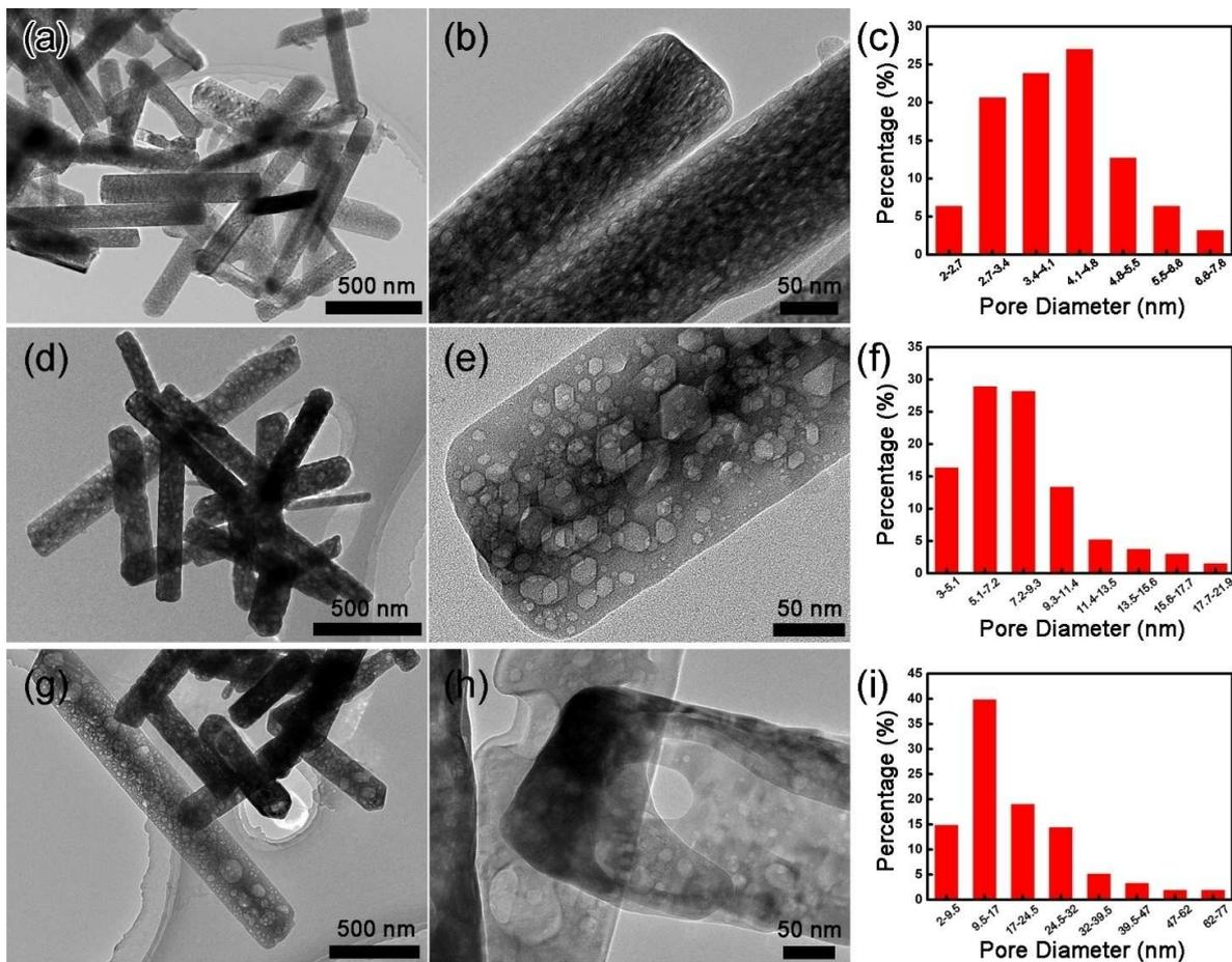
Figure 6. Typical TEM images of Fe<sub>2</sub>O<sub>3</sub>-400 (a, b), Fe<sub>2</sub>O<sub>3</sub>-500 (d, e), Fe<sub>2</sub>O<sub>3</sub>-600 (g, h). (c, f, i) the corresponding size distribution of the pores in Fe<sub>2</sub>O<sub>3</sub> nanorods.
