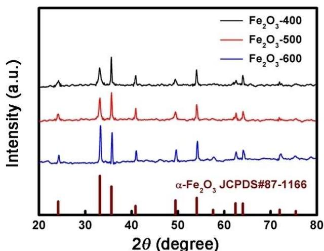
Figure 2. XRD patterns of annealed product at different temperatures.
