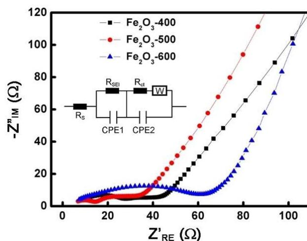
Figure 9. EIS of  $\text{Fe}_2\text{O}_3$ -400,  $\text{Fe}_2\text{O}_3$ -500 and  $\text{Fe}_2\text{O}_3$ -600 electrodes after 200 cycles, insert is the equivalent electrical circuit.
