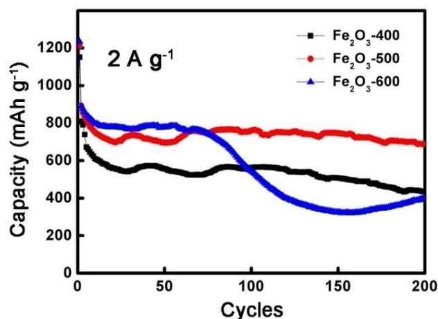
Figure 8. Cycling performances of  $\text{Fe}_2\text{O}_3$ -400,  $\text{Fe}_2\text{O}_3$ -500 and  $\text{Fe}_2\text{O}_3$ -600 at  $2 \text{ A g}^{-1}$ .
