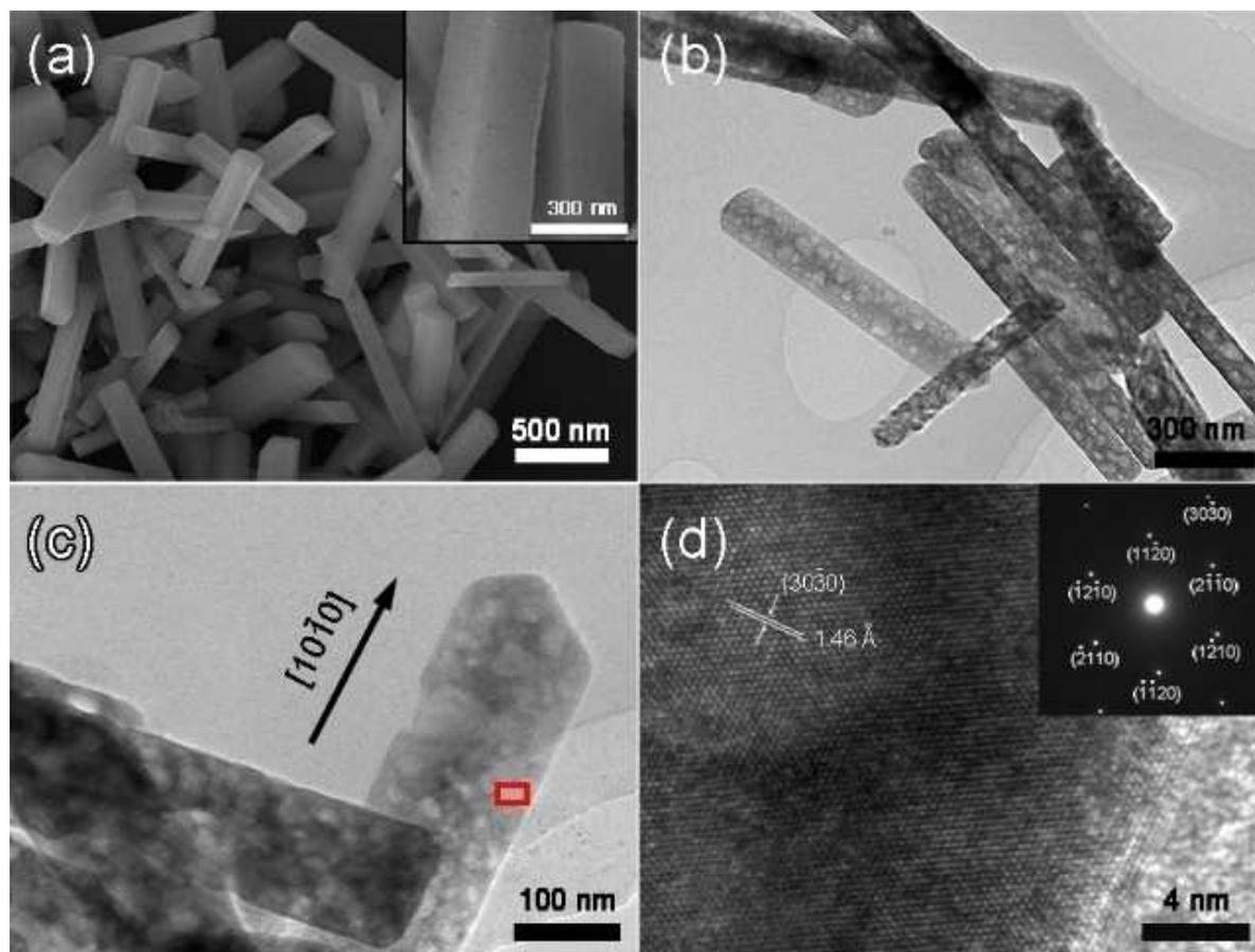
**Figure 4.** (a) Typical SEM image of  $\text{Fe}_2\text{O}_3$ -500, inset is magnified SEM image. (b, c) Bright-field (BF) TEM images of  $\text{Fe}_2\text{O}_3$ -500. (d) HRTEM image taken from the region enclosed by a red rectangle, inset is the corresponding SAED pattern.
