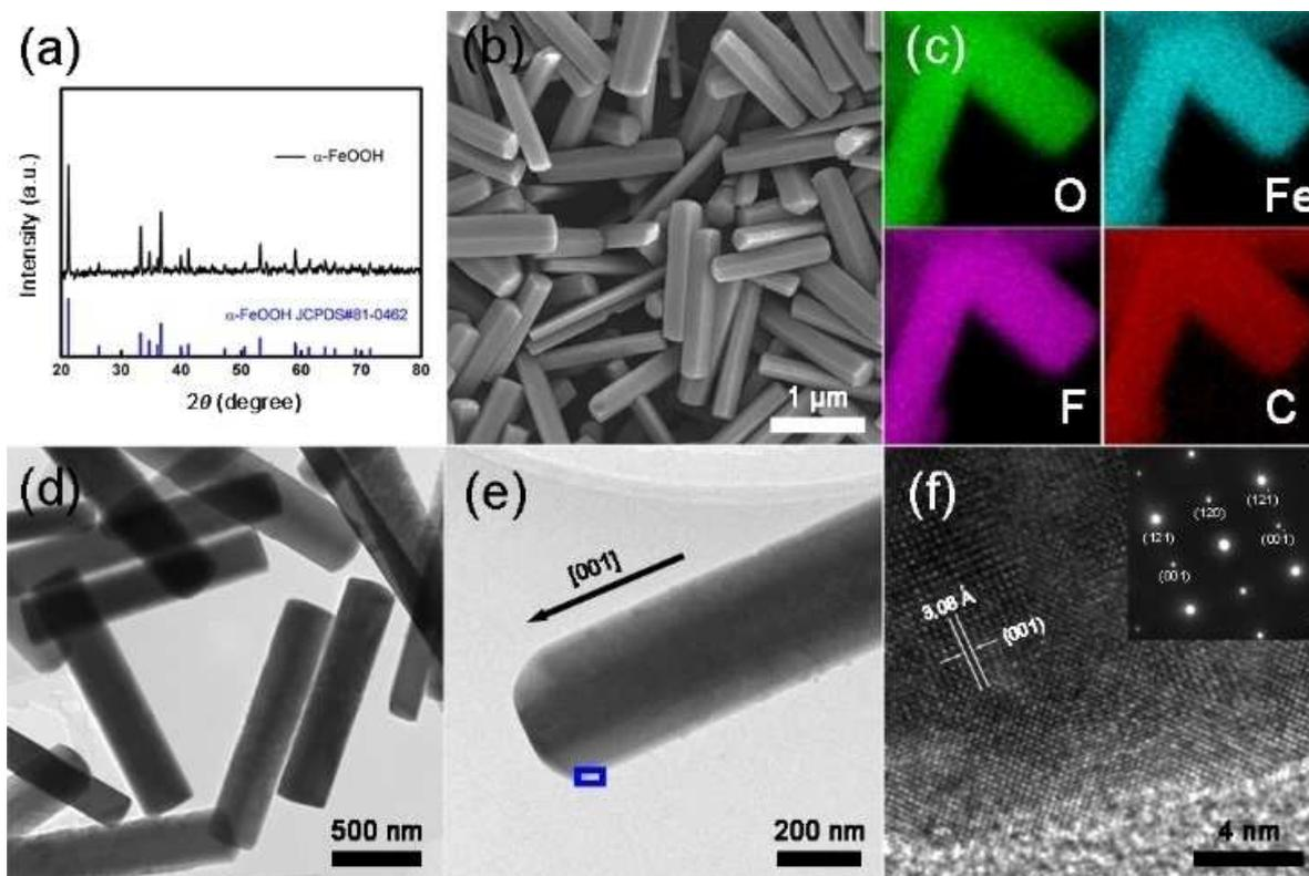
**Figure 1.** (a–c) XRD pattern, SEM image and element mapping of precursors. (d–e) typical TEM images of precursors. (f) HRTEM image taken from (e). Inset in (f) is the corresponding SAED pattern.
