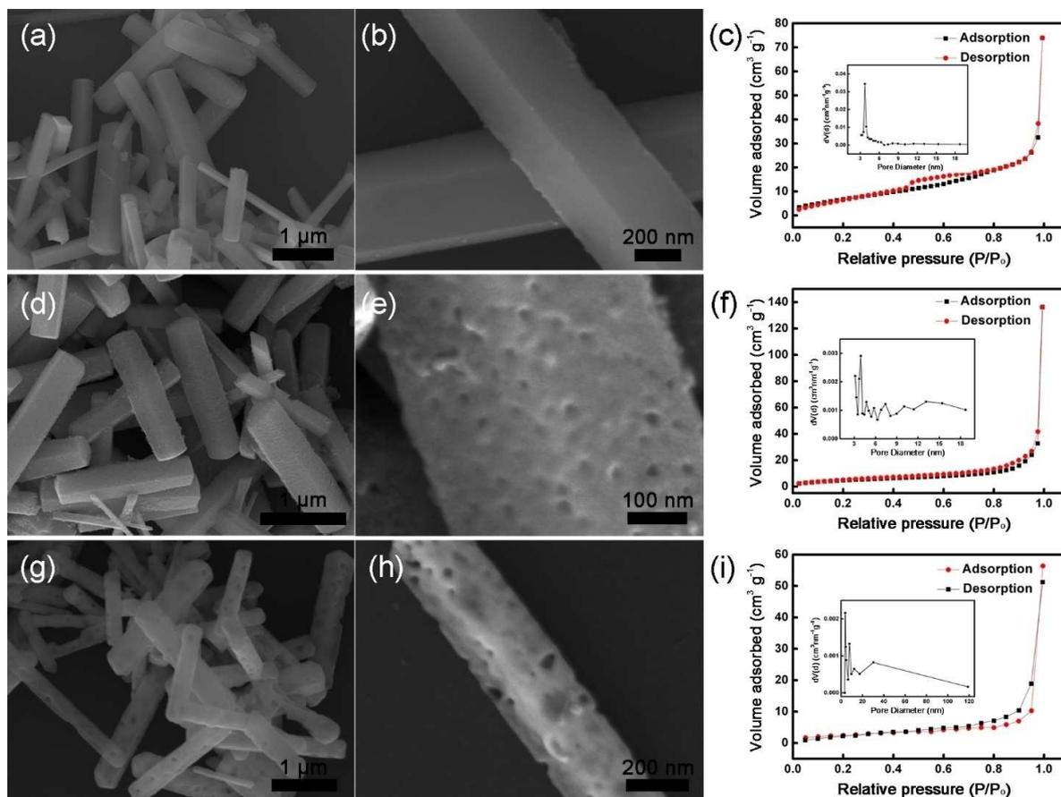
**Figure 5.** Typical SEM images and Nitrogen adsorption-desorption isotherms of (a-c)  $\text{Fe}_2\text{O}_3$ -400 nanorods, (d-f)  $\text{Fe}_2\text{O}_3$ -500 nanorods, and (g-i)  $\text{Fe}_2\text{O}_3$ -600 nanorods.
