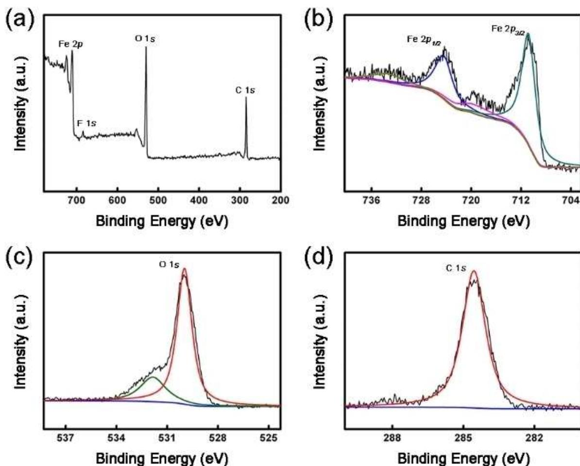
Figure 3. XPS spectra for the Fe<sub>2</sub>O<sub>3</sub>-500. (a) full scan; (b) Fe 2*p*; (c) O 1s; (d) C 1s.
