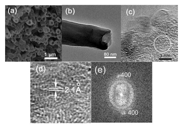
**Fig. 1.** (a) SEM images of the PA6 nanotube arrays; (b) a typical TEM image of PA6 nanotube; (c) HRTEM image of the sidewall in image (b); (d) enlarged view of marked area in (c); (e) FFT image of (c).
