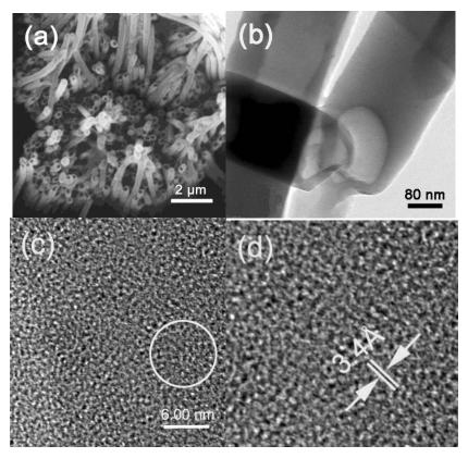
**Fig. 2.** (a) SEM image of PS nanotube arrays; (b) TEM image of PS nanotubes; (c) HRTEM image of the sidewall in image (b); (d) enlarged view of marked area in (c).
