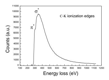
Fig. 5. A typical EELS spectrum taken from one of PS nanotubes.
