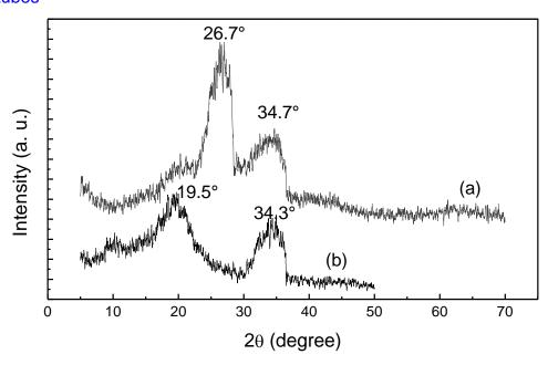
Fig. 4. XRD spectra of polystyrene: (a) PS nanotubes; (b) bulk PS.
