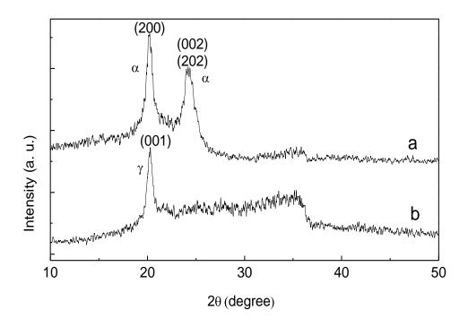
Fig. 3. XRD spectra of polyamide 6: (a) bulk PA6; (b) PA6 nanotubes.
