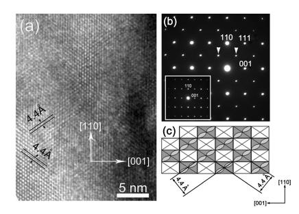
FIG. 3. (a) HRTEM image of BCMO film with a thickness of 200 nm at 103 K. (b) SAED pattern taken from the BCMO film in (a) at 103 K. Inset shows a typical SAED pattern taken at the room temperature. (c) Schematic model for the CO behavior in the BCMO film.
