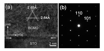
FIG. 1. HRTEM images and SAED patterns taken from thinner films at 103 K, (a) and (b) film thickness is 40 nm.
