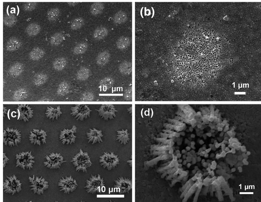
**Fig. 1** – SEM images of patterned AAO templates and Cu nanowire arrays: (a) Patterned AAO template with circular patterns; (b) An enlarged pattern in panel (a); (c) SEM image of Cu nanowire arrays with circular patterns; and (d) An enlarged SEM image of the pattern in panel (c).
