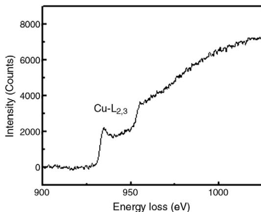
**Fig. 4 – EELS spectrum of Cu nanowires.**
