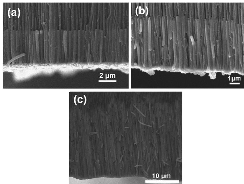
**Fig. 2** – SEM images of the Cu nanowire with different deposition time: (a) 5 min; (b) 10 min; and (c) 20 min.
