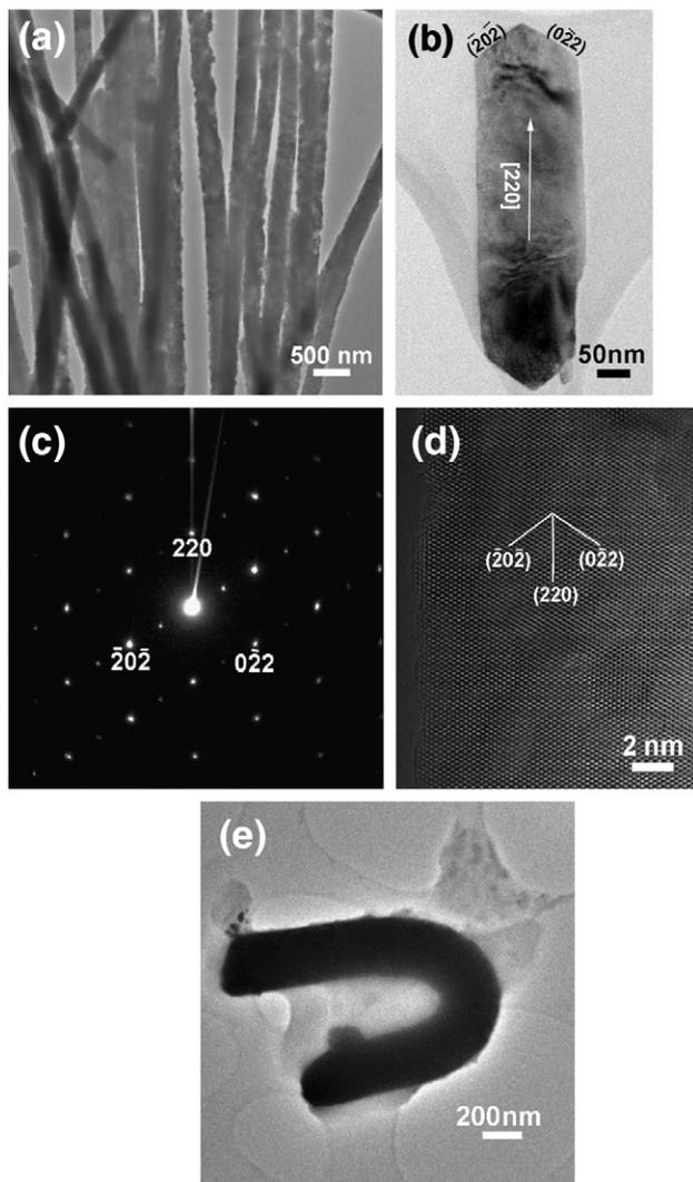
**Fig. 3 – (a) TEM image of Cu nanowires; (b) TEM image of a randomly-selected Cu wire; (c) SAED pattern taken from (b); (d) HRTEM image of Cu nanowire shown in (b); and (e) TEM image of a bent nanowire.**
