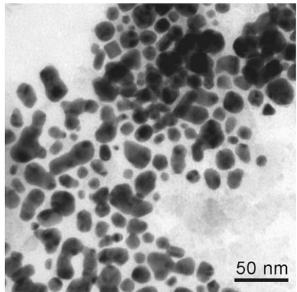
**Fig. 5** A typical low-magnification TEM image of the gold nanoparticles after the annealing at 200 °C for 60 min
