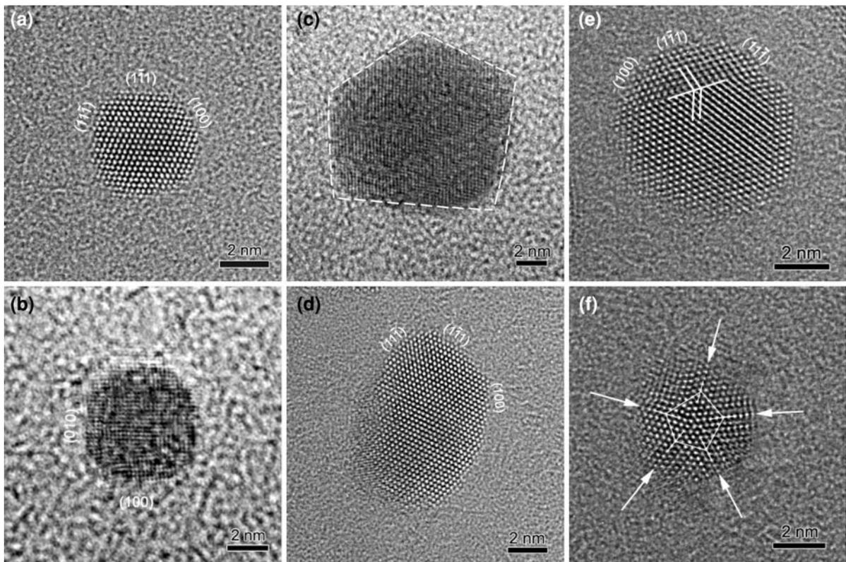
**Fig. 2** HRTEM images of gold nanoparticle with facets, **a–c** regular shapes: **a** a hexagon; **b** a square; **c** a pentagon; and **d** an elongated shape; **e** a particle with a single-twin configuration; **f** particle with a fivefold twinning configuration
